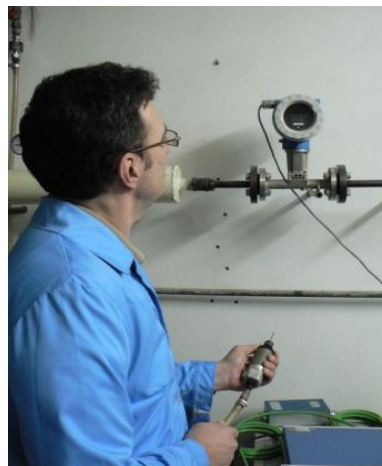
Measuring air consumption idling
