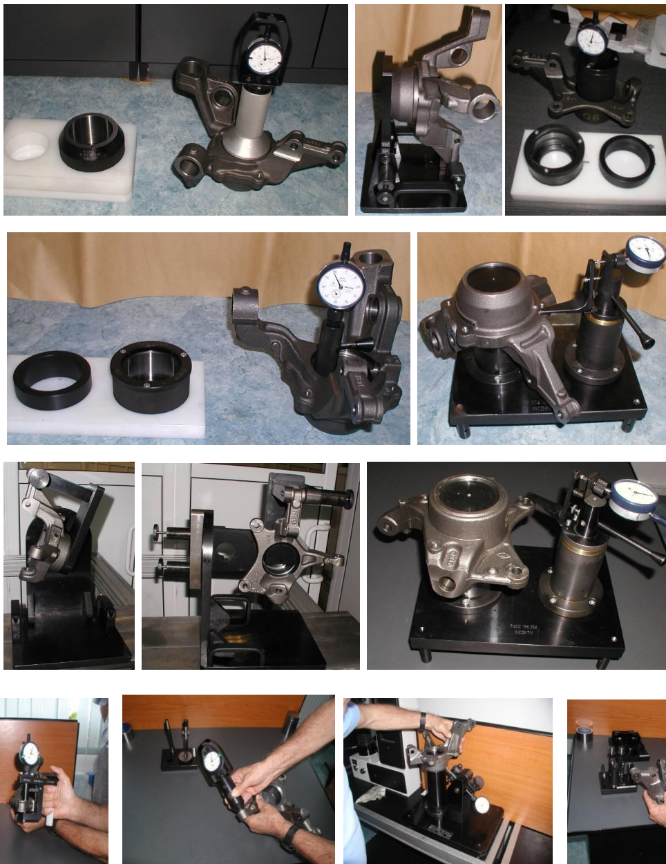
Device for thickness control of axle pin base arm
